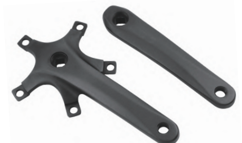
MODEL : LI201 HBK LENGTH:165-170MM BCD:130MM
